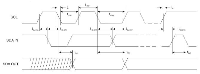
Figure 6-3. Write Cycle Timing
