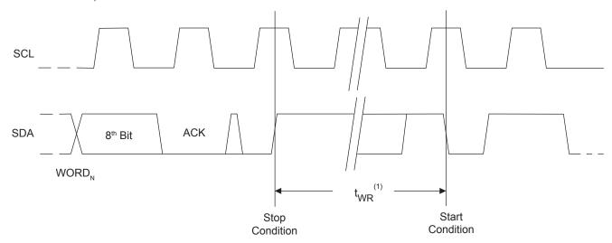
Notes: 1. The write cycle time  $t_{WR}$  is the time from a valid Stop condition of a write sequence to the end of the internal clear/write cycle.
