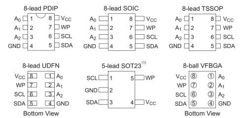
Note: 1. For use of 5-lead SOT23, the software A2, A1, and A0 bits in the device address word must be set to zero to properly communicate.
